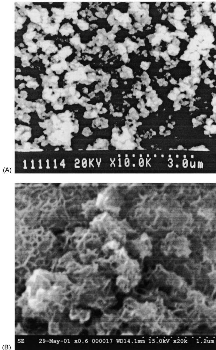
Fig. 4. SEM micrograph of NiB amorphous alloys (A: NiB-1; B: NiB-2).
