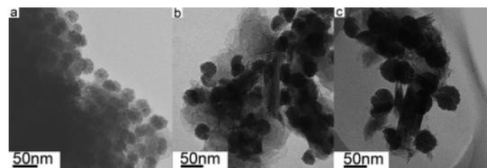
**Figure 3.** TEM images of supported amorphous Ni-B catalysts, prepared using different en/Ni<sup>2+</sup> with the same pH value, with particle sizes of (a) Ni-B<sub>2-13.6</sub>, 25 ± 1.1 nm, (b) Ni-B<sub>4-13.6</sub>, 41 ± 1.4 nm, and (c) Ni-B<sub>8-13.6</sub>, 50 ± 1.4 nm.
