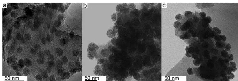
**Figure 1.** TEM images of series-supported amorphous Ni-B<sub>3-y</sub> catalysts, prepared using a different pH value, with particle sizes of (a) Ni-B<sub>3-12.8</sub>, 16 ± 1.2 nm, (b) Ni-B<sub>3-13.2</sub>, 33 ± 1.5 nm, and (c) Ni-B<sub>3-13.6</sub>, 36 ± 1.4 nm.
