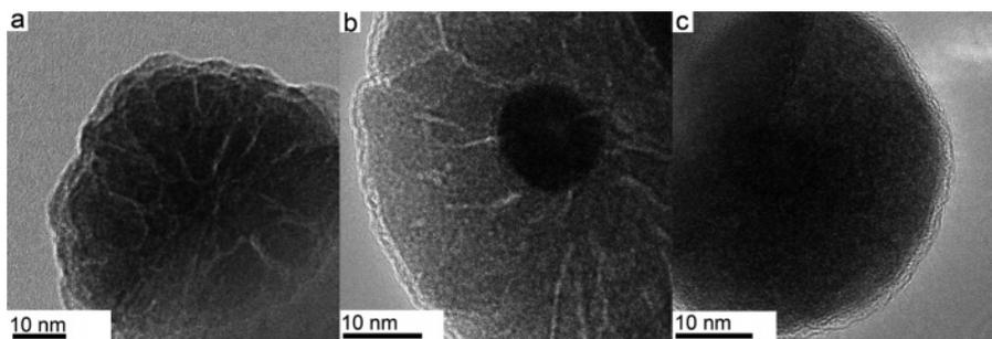
Figure 6. HRTEM images of supported Ni-B catalysts. (a) Ni-B<sub>3-13.6</sub>; (b) Ni-B<sub>3-13.6-2(Pb)</sub>; and (c) Ni-B<sub>3-13.6-2(Pb)</sub>.
