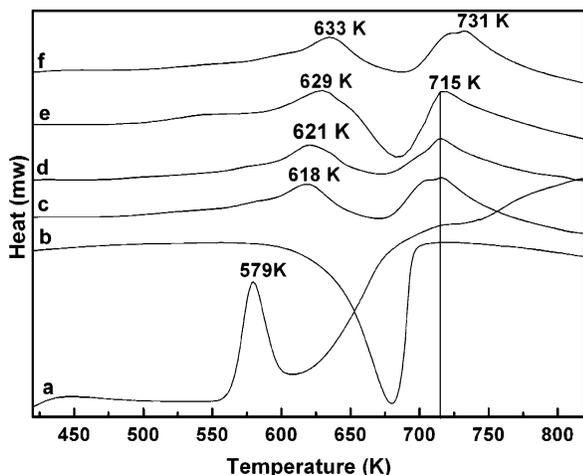
**Figure 5.** DSC curves of the specimens (a) unsupported Ni-B<sub>3-13.6</sub>, (b) Ag/MgO support, (c) Ni-B<sub>2-13.6</sub> with 8.2 wt % nickel loading, (d) Ni-B<sub>3-13.6</sub> with 15.5 wt % nickel loading, (e) Ni-B<sub>3-13.6</sub> with 8.5 wt % nickel loading, and (f) Ni-B<sub>4-13.6</sub> with 7.7 wt % nickel loading.
