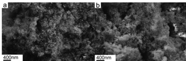
**Figure 4.** SEM images of the specimens (a) Ni-B<sub>3-13.6</sub> with 8.5 wt % nickel loading and (b) Ni-B<sub>3-13.6</sub> with 15.5 wt % nickel loading.
