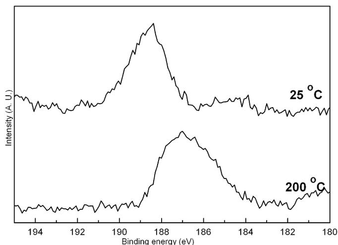
**Fig. 5.** XPS spectra of B 1s for Pd/Ni-B treated at different temperatures in a 40-ml/min  $N_2$  flow.
