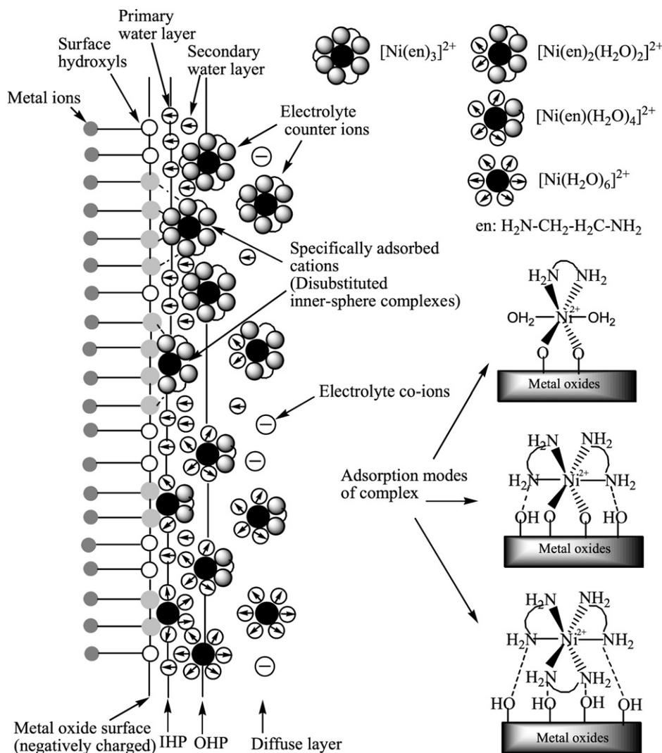
**Fig. 5.** A schematic illustration of the electrical double layer between the surface of metal oxides and the plating solution and the adsorption modes of nickel complexes. By IHP we symbolize the so-called inner Helmholtz plane, and by OHP the so-called outer Helmholtz plane. For simplicity we use the term “surface hydroxyls” to describe unprotonated or singly or doubly protonated surface oxygen, and we consider only singly coordinated surface oxygen.
