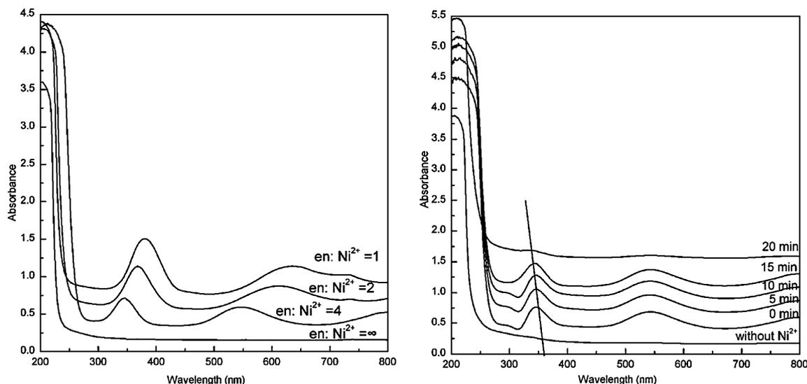
**Fig. 6.** (a) UV-vis spectra of  $[\text{Ni}(\text{en})_x(\text{H}_2\text{O})_{(6-2x)}]^{2+}$  in the aqueous solutions prepared with different nominal  $\text{en}/\text{Ni}^{2+}$  ratios; and (b) UV-vis spectra of  $[\text{Ni}(\text{en})_x(\text{H}_2\text{O})_{(6-2x)}]^{2+}$  in the plating solution prepared with nominal  $\text{en}/\text{Ni}^{2+}$  ratio of 4 at different plating times.
