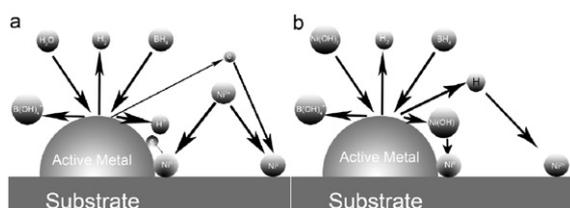
**Fig. 7.** Processes of nickel deposition on substrates based on (a) the electrochemical mechanism and (b) the hydrolyzed nickel mechanism.
