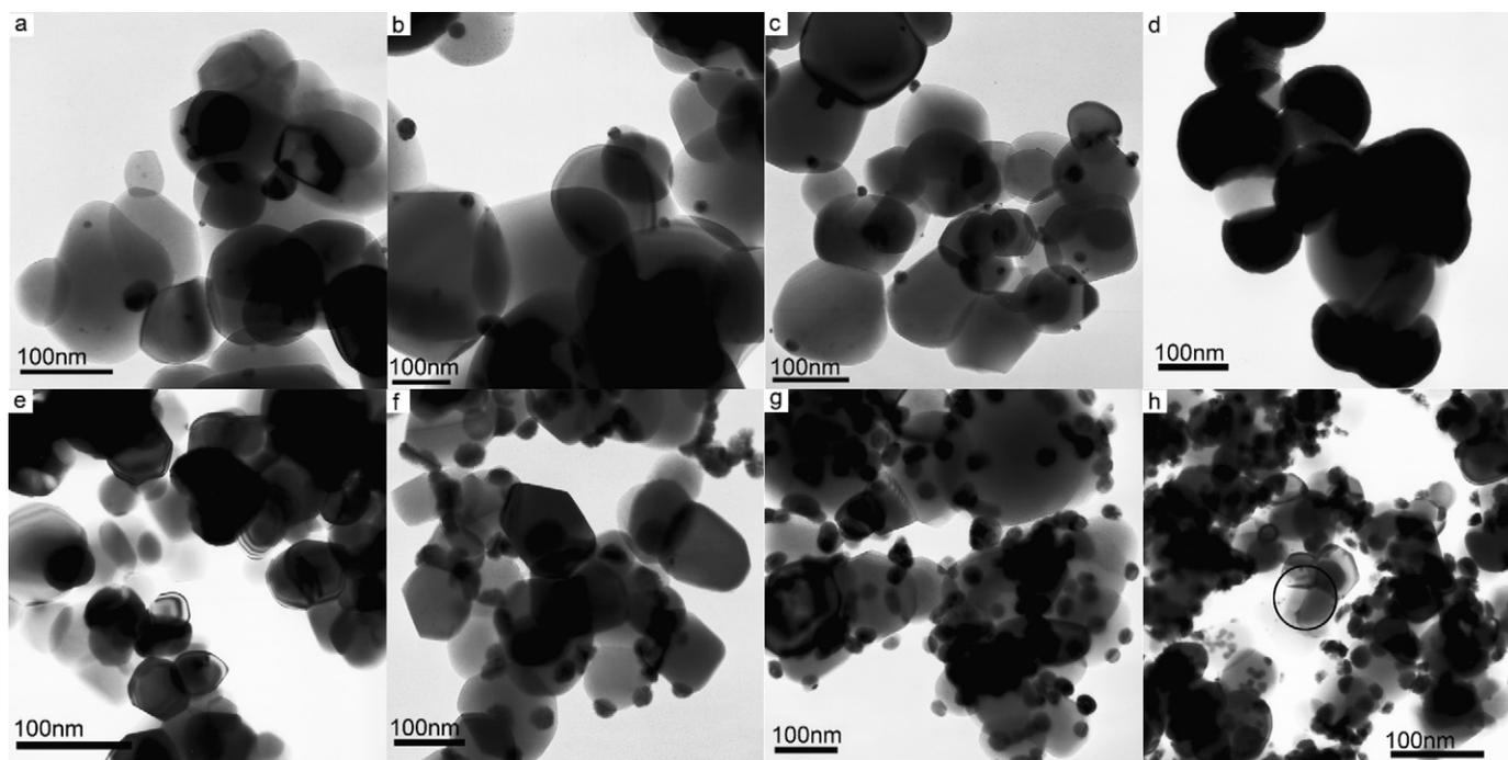
**Fig. 3.** TEM images of samples with different Ag weight loadings. Ag/TiO<sub>2</sub>: (a) 0.02%, (b) 0.05%, and (c) 0.16%. Ni/TiO<sub>2</sub>: (d) 0.02%, (e) 0.02%, (f) 0.05%, (g) 0.1%, and (h) 0.16%.
