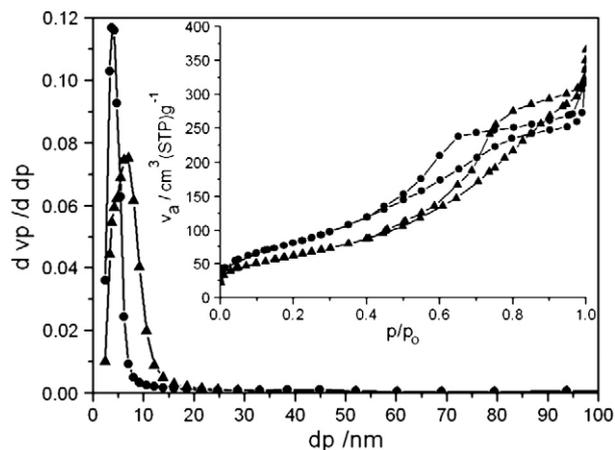
**Fig. 3.** N<sub>2</sub> adsorption–desorption isotherms and pore size distributions of samples: ▲ sample A; ● sample B.
