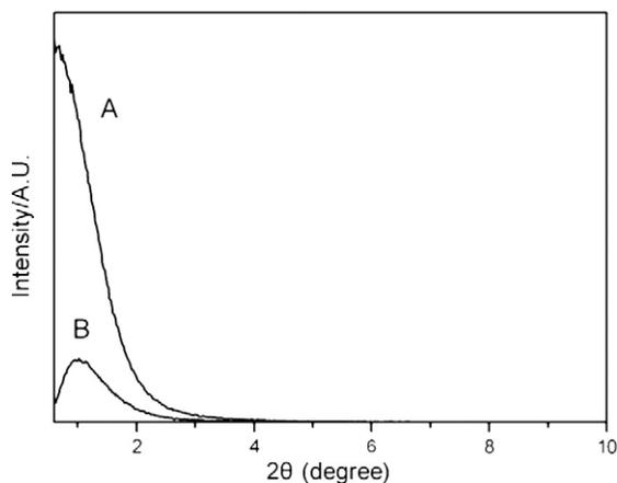
**Fig. 1.** Small-angle XRD patterns of MA after calcination at 600 °C: A (concentration of surfactant of 0.1 mol/L), B (concentration of surfactant of 0.4 mol/L).
