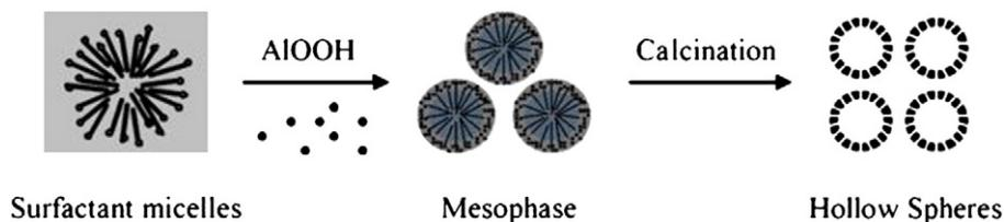
**Scheme 1.** Schematic illustration for the formation process of the hollow alumina mesoporous nanospheres.
