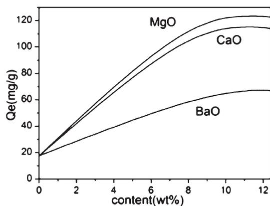
**Fig. 3** Effect of different concentrations of modifier (adsorption conditions: initial Cd<sup>2+</sup> concentration = 250 ppm, contact time = 2 h, pH = 7, temperature = 298 K, adsorbent dose = 2 g L<sup>-1</sup>).
