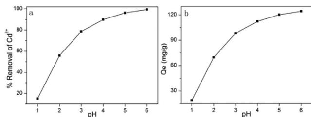
Fig. 10 Effect of pH on the adsorption of  $\text{Cd}^{2+}$  onto MM. (a) The percentage removal of  $\text{Cd}^{2+}$  of different pH. (b) The adsorption amount of different pH (adsorption conditions: initial  $\text{Cd}^{2+}$  concentration =  $250 \text{ mg L}^{-1}$ , adsorbent dose =  $2 \text{ g L}^{-1}$ , contact time = 2 h, temperature = 298 K).
