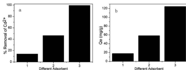
**Fig. 5** The adsorption capacity of different adsorbents. (a) The percentage removal of Cd<sup>2+</sup> of different adsorbents. (b) The adsorption amount of different adsorbents. (1) MCM-41, (2) MgO, (3) MM (adsorption conditions: initial Cd<sup>2+</sup> concentration = 250 ppm, contact time = 2 h, pH = 7, temperature = 298 K, adsorbent dose = 2 g L<sup>-1</sup>).
