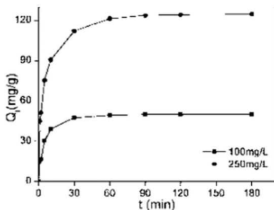
Fig. 6 Adsorption kinetics data for adsorption of  $\text{Cd}^{2+}$  on MM (adsorption conditions: adsorbent dose =  $2 \text{ g L}^{-1}$ , pH = 7, temperature =  $298 \text{ K}$ , contact time = 2 h).
