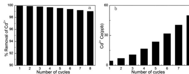
Fig. 11 (a) The percentage removal of  $\text{Cd}^{2+}$  of different cycles. (b) The equilibrium liquid phase concentrations of  $\text{Cd}^{2+}$  of different cycles. Regenerated use of MM adsorbent for the removal of  $\text{Cd}^{2+}$  (adsorption conditions: initial  $\text{Cd}^{2+}$  concentration =  $5 \text{ mg L}^{-1}$  (5000 ppb), contact time = 2 h, pH = 7, temperature = 298 K).
