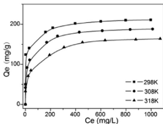
**Fig. 8** Adsorption isotherm data for adsorption of Cd<sup>2+</sup> on MM at different temperatures (adsorption conditions: adsorbent dose = 2 g L<sup>-1</sup>, contact time = 2 h, pH = 7).
