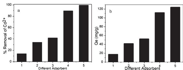
**Fig. 2** The adsorption capacity of different adsorbents. (a) The percentage removal of Cd<sup>2+</sup> of different adsorbents. (b) The adsorption amount of different adsorbents. (1) MCM-41, (2) Activated carbon, (3) BM, (4) CM, (5) MM (adsorption conditions: pH = 7, temperature = 298 K, contact time = 2 h, initial Cd<sup>2+</sup> concentration = 250 mg L<sup>-1</sup>, adsorbent dose = 2 g L<sup>-1</sup>).
