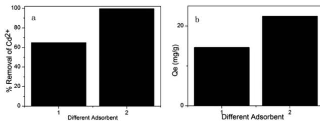
**Fig. 4** The adsorption capacity of different adsorbents. (a) The percentage removal of Cd<sup>2+</sup> of different adsorbents. (b) The adsorption amount of different adsorbents. (1) AC-Mg, (2) MM (adsorption conditions: initial Cd<sup>2+</sup> concentration = 45 ppm, contact time = 2 h, pH = 7, temperature = 298 K, adsorbent dose = 2 g L<sup>-1</sup>).
