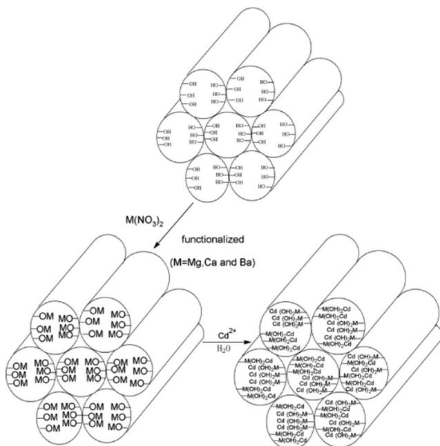
Scheme 1 Schematic mechanism for  $\text{Cd}^{2+}$  adsorption.
