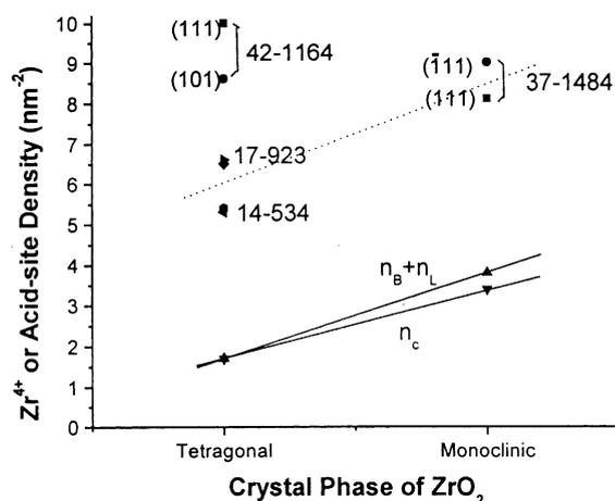
Fig. 6.  $\text{Zr}^{4+}$  density and acid-site density of tetragonal and monoclinic  $\text{ZrO}_2$ . The texts on the left of points are the Miller indexes, the right-side text the JCPDS No.,  $n_B + n_L$  the density of total acid sites calculated from IR data,  $n_C$  the density of total acid sites determined by  $\text{NH}_3$ -adsorption measurements.
