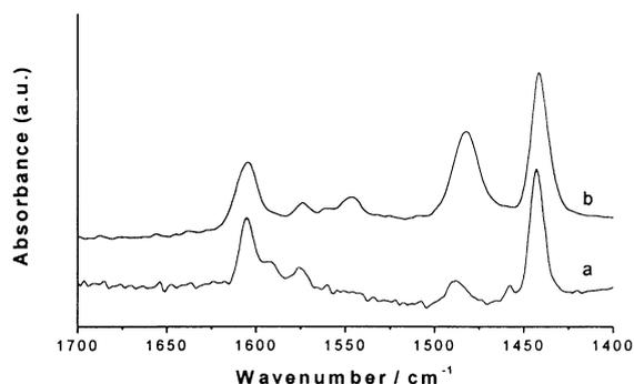
Fig. 5. IR spectra after pyridine adsorption of (a) TZ50 and (b) MZ96.
