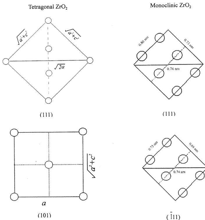
Fig. 4.  $\text{Zr}^{4+}$  array in different planes of tetragonal and monoclinic (JCPDS No.37-1484)  $\text{ZrO}_2$ .
