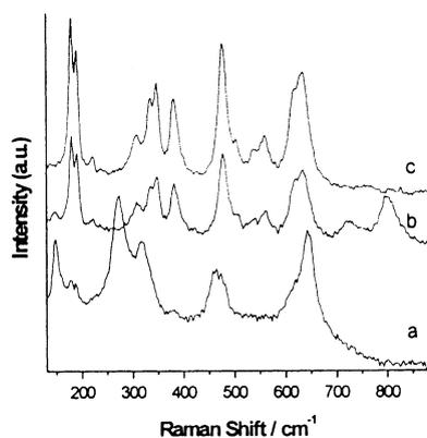
Fig. 3. Raman spectra of (a) TZ50, (b) MZ50 and (c) MZ96.
